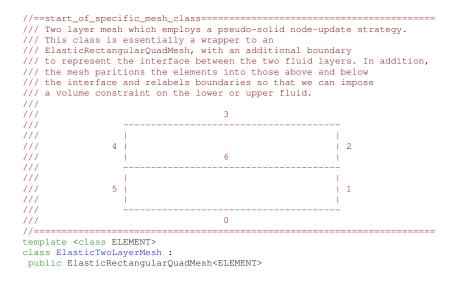
The arguments to the constructor specify the number of elements in the horizontal direction and in each layer and also the width of the container and the height of each layer. The remaining arguments determine whether the mesh should be made periodic in the x direction and are the TimeStepper object.
